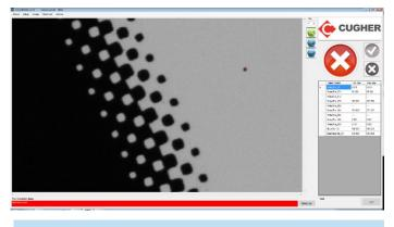
The proposed solution involves the use of two highresolution monochromatic linear cameras, each with 16,384 pixels. These digital cameras scan the printed glass line by line as it moves along the conveyor. The complete image of the glass can be captured in just 0.6 seconds, depending on the conveyor's speed.
