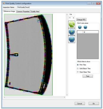
Training an inspection setup involves configuring the print quality control after generating the overall model of the glass. The glass surface is automatically divided into small sections based on the detected patterns, which include printed designs, solid black greas, and clear glass regions.
