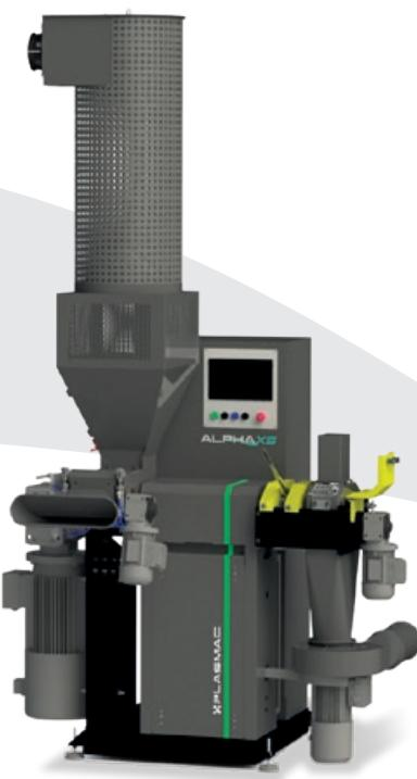
The **ALPHA XS** recycling extruder uses Plasmac's unique Short Screw Technology (S.S.T.), which is based around a dual diameter 10:1 L/D ratio screw.
